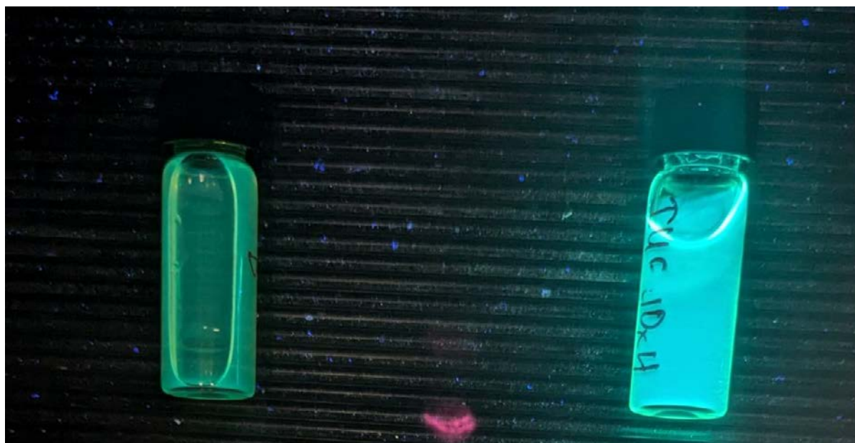
Figure 2. Mixture of DMA and CA monomers (on the left) and a poly(DMA-co-CA) copolymer (on the right) under UV-light.
